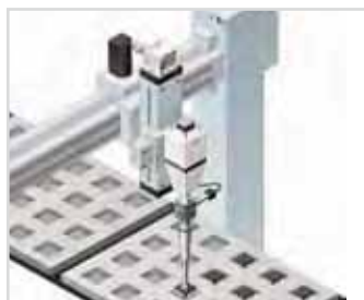
Confirming suction of electronic component
